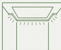
False Ceiling with LED Cove Lighting
